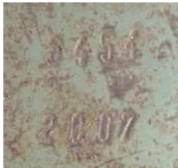
Serial number "3454" on the base plate and "2007" as the year of fabrication
